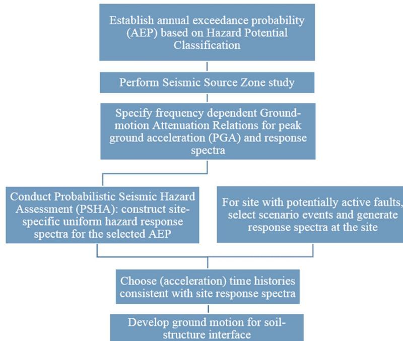
Figure 1. LRIA Process to assess seismic safety of a dam [4]
